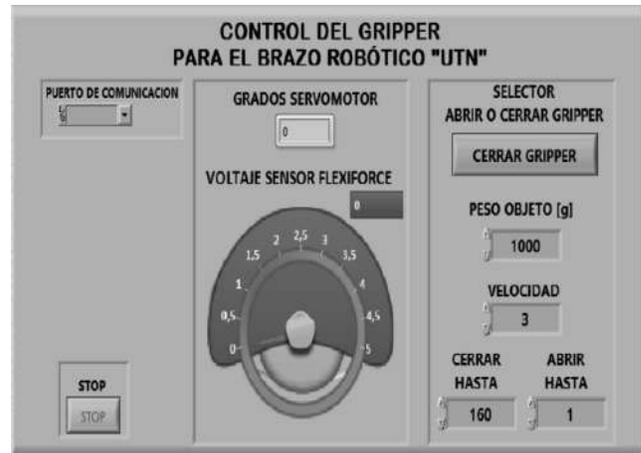
**Figura 9.** Interfaz principal del control del Gripper
