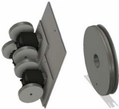
Fig. 3. Simulation of the mechanic system for the active orthosis. a) Polleys coupled to the servomotors. b) Polley
