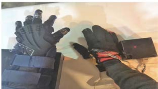
Fig. 6 Robotic system for bilateral rehabilitation of the left hand
